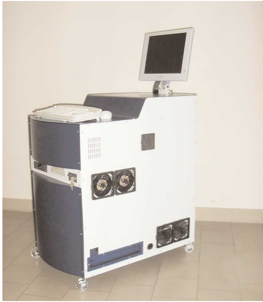
Figure 1 - The MOBILE Dual-pulse Instrument (Modi) used for LIBS analysis
