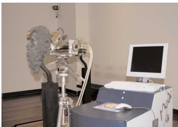
Figure 1 – The Modi LIBS instrument during the measurements at Museum of Magna Grecia
