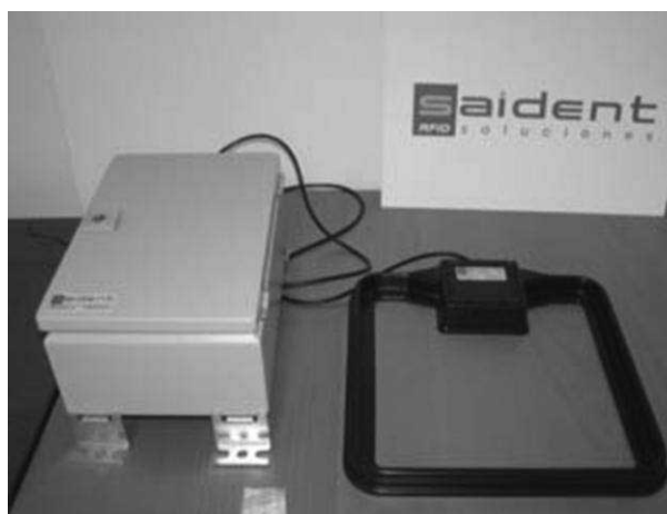
Figure 5: A RFID reader (left) and its antenna
